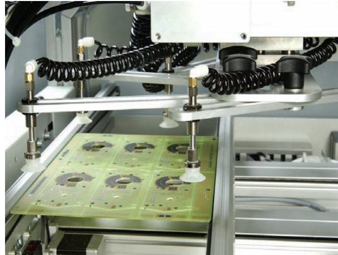
Springloaded vacuum cradle assembly
