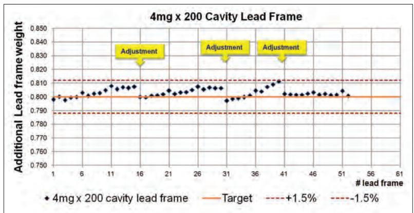
**Figure 3:** Dispensing weight adjustment with CPJ+.
