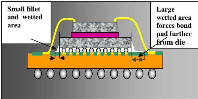
**Figure 2: Flip chip on bottom of stack**
