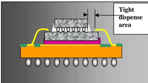
**Figure 3: Flip chip on top of stack**
