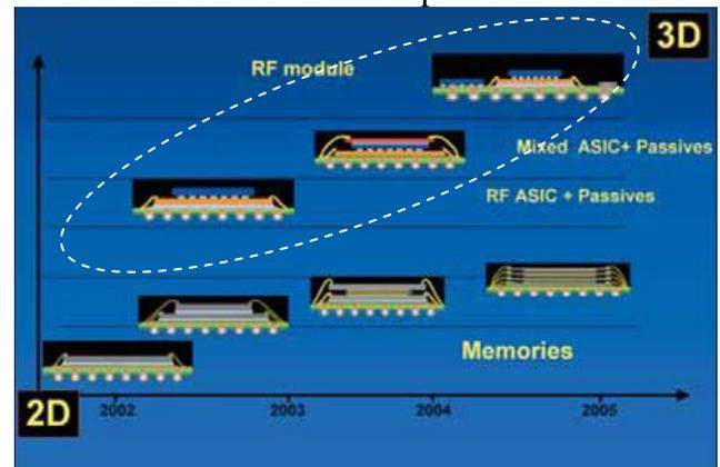
**Figure 1: Ball Grid Array (BGA), from the "single chip" version to multiple stacks and Modules (REF 1)**
