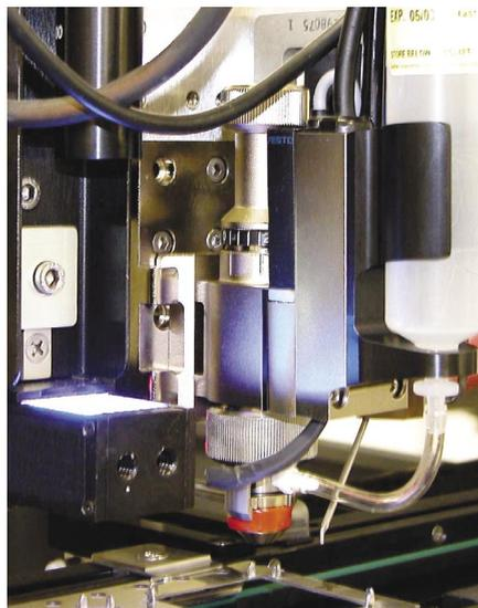
**Figure 1.** A pneumatic piston impels fluid through a narrow orifice at the end of the nozzle.
