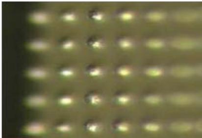
**Figure 5.** Pre-applied underfill by spray coating
