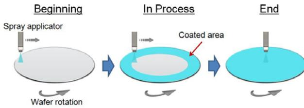
**Figure 4.** Spray coating process flow chart
