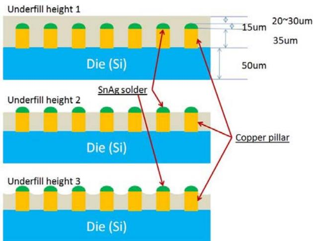
**Figure 1.** Pre-applied underfill shapes with different volume
