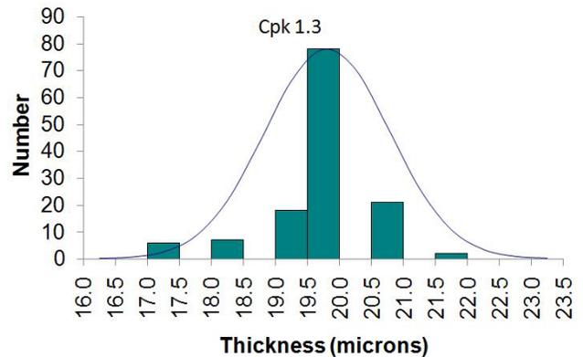
Figure 10. Spray coating thickness distribution for wafers.
