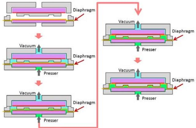
**Figure 2.** Vacuum lamination process flow chart
