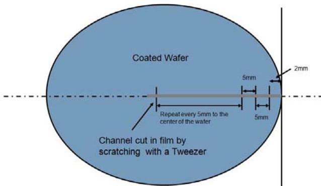
Figure 8. Coating thickness measurement method diagram
