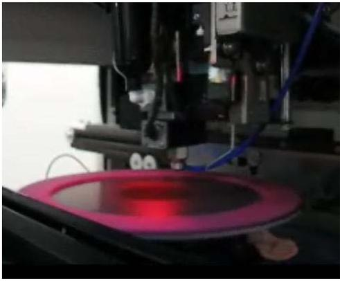
Figure 7. 300mm wafer that has been coated
