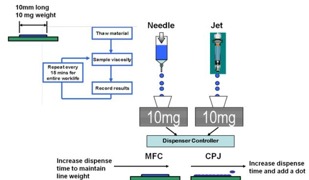
**Figure 6 Mass Flow Calibration principle**
